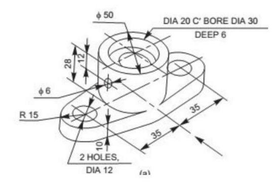
Figure 1: Dimensioning of bearing housing
